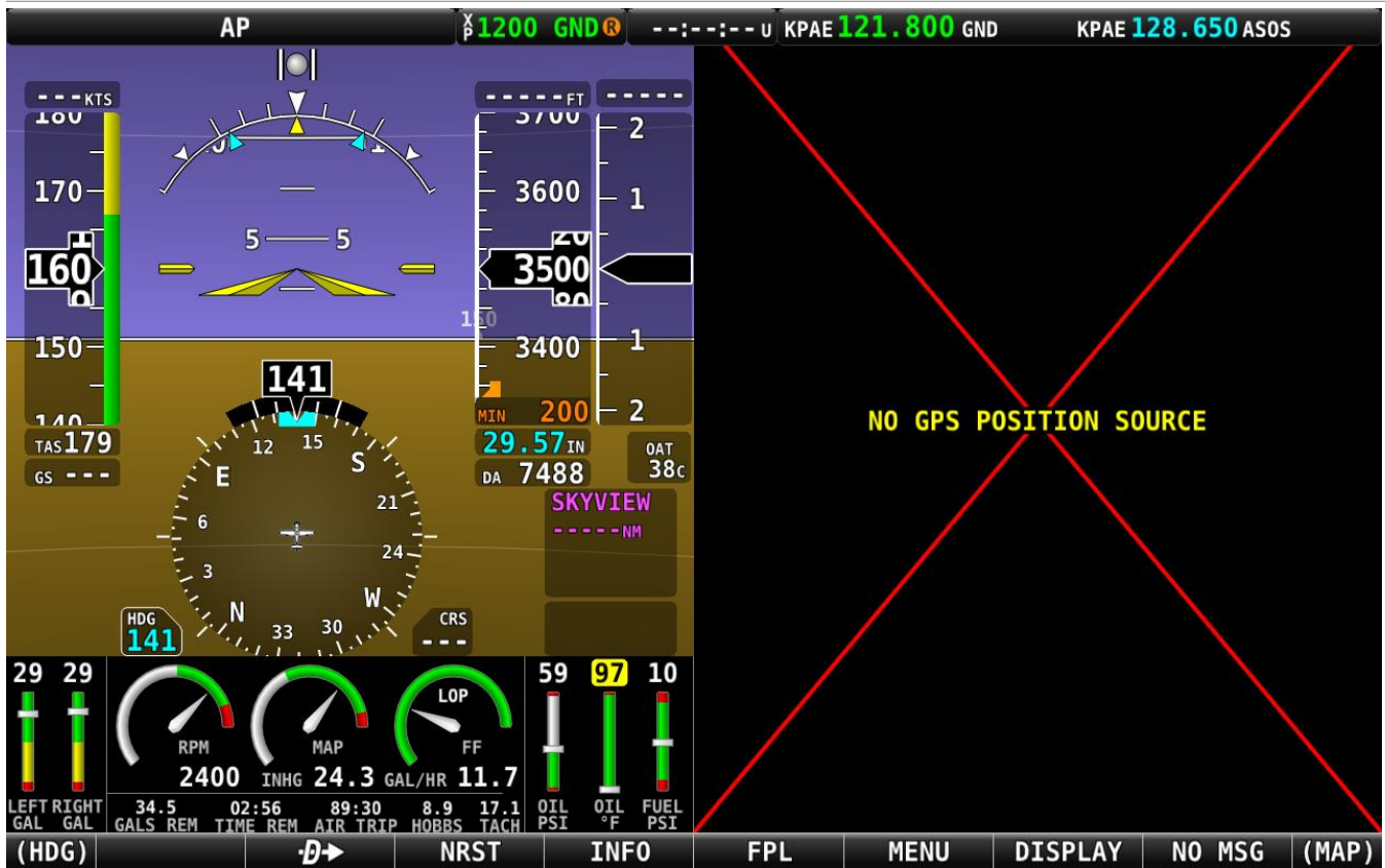
Figure 40: Example of GPS Antenna/Receiver Failure
