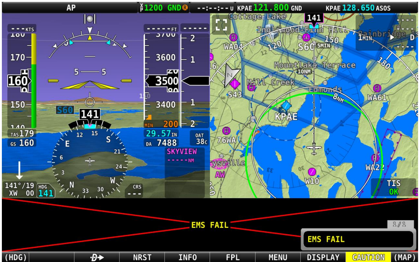
Figure 41: Example of EMS Module Failure
