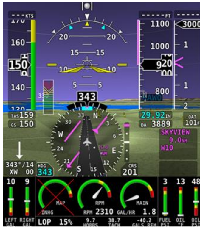
Figure 42: Example of an EMS Sensor Failure
